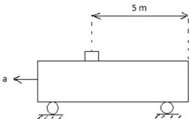
1. A block of mass 10 kg is placed at a distance of 5 m from the rear end of a long trolley as shown. The coefficient of friction between the block and the surface below is 0.2 Starting from rest the trolley is accelerated uniformly with a = 3  $ms^{-2}$  At what distance from the starting point will the block fall off the trolley. Take g = 10  $ms^{-2}$  \*a) 15 m b) 20 m c) 25 m d) 30 m
