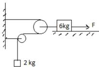
3. The system starts from rest and 6 kg block attains a velocity of 5 m/s after it has moved 5 m towards the right. Assuming all surfaces are frictionless and pulleys and strings are light, the value of F is
