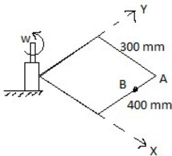
1. The rectangular plate is rotating about an axis passing through its corner and perpendicular to its plane with angular velocity  $w = 10 \text{ rad/s}$ .
