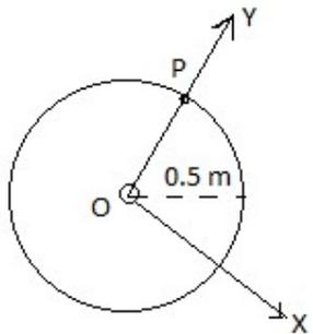
2. The circular disc rotates about its centre O in the clockwise direction. At a certain instant the point P on the rim has an acceleration  $\vec{a} = -3\hat{i} - 4\hat{j}$  m/s<sup>2</sup>. For that instant
