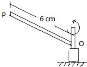
3. The rod starts from rest and acquires a speed of 60 rev/min in 2 sec. by rotating in the horizontal plane about the vertical axis shown with a constant angular acceleration.
