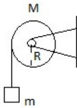
5. A uniform disc of radius  $R$  and mass  $M$  is free to rotate about a fixed axis perpendicular to its plane and passing through its centre. A string is wrapped over its rim and a block of mass  $m$  is attached to the free end of the string as shown. The block is released from rest. If the string does not slip on the rim, find the acceleration of the block. Neglect the mass of the string.
