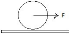
43. A solid sphere of mass 2 kg is pulled by a constant horizontal force through its centre on a rough horizontal surface with  $\mu = 0.5$ . The maximum value of  $F$  so that the sphere rolls without slipping is ( $g = 10 \text{ ms}^{-2}$ )
