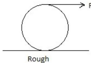
14. A ring of mass m and radius R is kept on a rough surface with a horizontal force F applied as shown. It rolls without slipping on the surface. Find the work done by the force F when the centre of mass moves a distance S.
