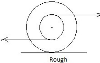
13. A spool is pulled horizontally by two equal and opposite forces as shown. Which of the following statements is correct?
