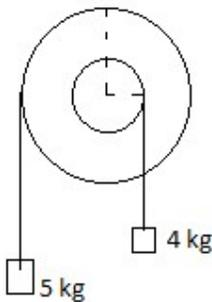
7. The M.I of the pulley system is  $4 \text{ kgm}^2$ . The radii of bigger and smaller pulleys are 2 m and 1 m respectively. The angular acceleration of the system is (in  $\text{rad/sec}^2$ )
