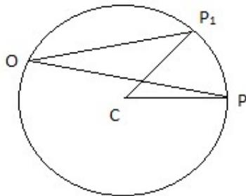
If a particle P is moving in a circle, its angular velocity about the centre of the circle C that is  $\omega_c$  is 2 times the angular velocity about any point on the circumference of the circle that is  $\omega_o$ .
