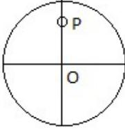
46. A disc of radius  $R$  rolls on a horizontal ground with linear acceleration  $a$  to the right and angular acceleration  $\alpha$  clockwise. It has a velocity  $v$  at the instant shown and angular velocity  $\omega$  also clockwise. What is the magnitude of the acceleration of the point  $P$ , distance  $r$  from the centre?
