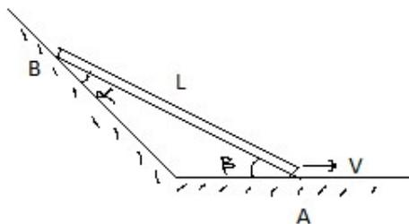
8. A rod of length  $L$  slides down along the inclined wall as shown. At the instant shown in the figure, the speed of the end A is  $v$ . What is the speed of B?
