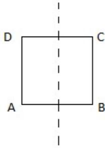
22. Four thin metal rods of mass  $m$  and length  $L$  each are welded to form a square ABCD as shown. What is the M.I of the composite structure about a line that bisects rods AB and CD and is in the plane of the structure?
