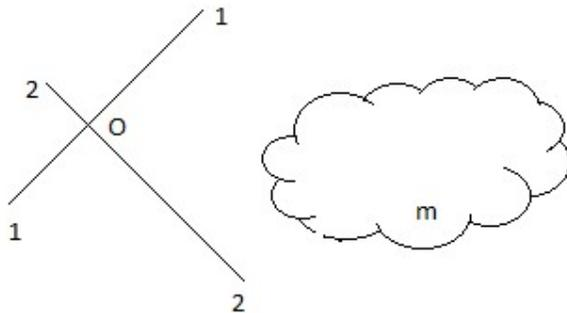
If the M.I of the plane lamina is known about axes 1-1 and 2-2 which are perpendicular to each other and in the plane of the lamina, their sum that is  $I_1 + I_2$  gives the M.I of the lamina about a third axis passing through the intersection of those two and perpendicular to them that is  $I_O$ .
