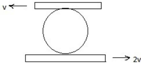
12. The disc of radius R is confined to roll without slipping while in contact with the two surfaces moving with velocities shown. What is the angular velocity of the disc?
