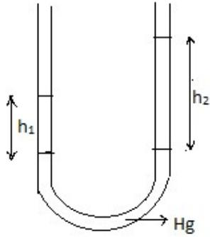
9. Water and oil are poured into two limbs of a U-tube containing mercury. The interfaces of mercury and the two liquids are at the same height in the two limbs. Determine the height  $h_1$  of water column if that of oil  $h_2 = 20$  cm. The density of oil is 0.9
