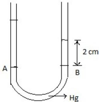
10. The liquids shown in the figure in the two arms are mercury and water. If the difference in heights of mercury column is 2 cm, find the height of  $h$  of water column.
