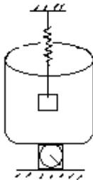
8. A beaker of mass 1 kg contains 2 kg of water and rests on a scale. A 2 kg block of aluminium (sp. gr. 2.7) suspended from a spring balance is submerged in water. Find the readings of both the scales.
